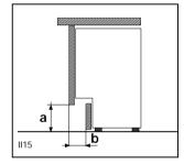
According to dimensions of (a) and (b) as shown on the figure, you will find on the following table the depth (x) of the cut to be made on the plinth.
